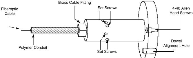
Figure 3 - Fiberoptic Feed Module
