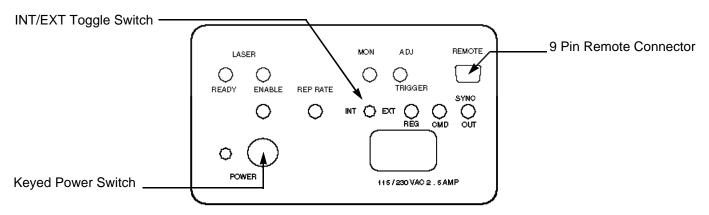
Figure 2 - Laser Control Panel
